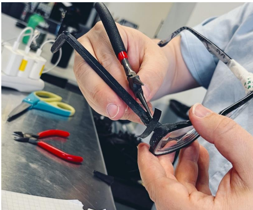
Mentor Adam demonstrating the installation of 3D printed glasses arm for a patron.
